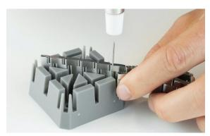
Rejoin the band by using a pin to join the remaining links and the buckle.
