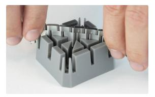
Detach the wristband from your Withings watch and place it on the base. The band has arrows indicating the direction in which the pin is to be pushed outward from the holes.
