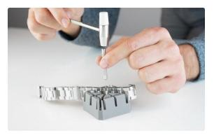
Use the small hammer to get the pushpin out of the wristband. Pull the pin from the other side when possible.
